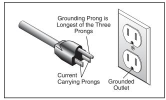
**Figure 2.** Typical 5-15 plug and receptacle.
